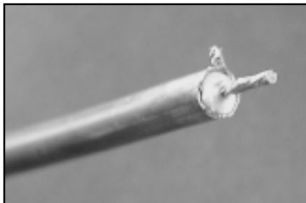
Figure 8—Feedpoint end of the Q section prior to final assembly.
